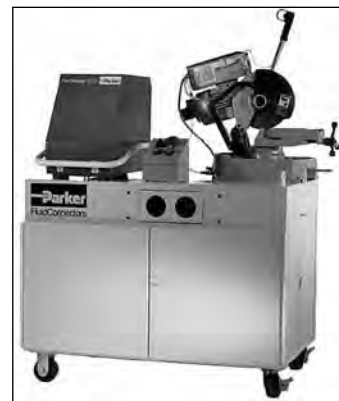
Fig. R135 — Tube Preparation Center TP1025
