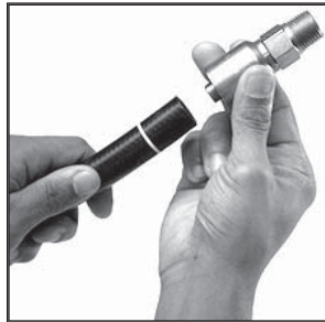
2. Push the hose all the way into the coupling to the insertion depth mark. Do not use lubricant to assemble spiral hose and fittings.
