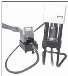
8. Reposition pusher, replace pin, operate pump until ring bottoms out on base plate.
