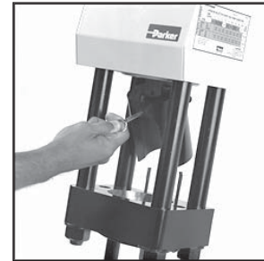
3. Remove pin from inside pusher unit so pusher will swing back. Lubricate the die bowl cavity to prevent wear.
