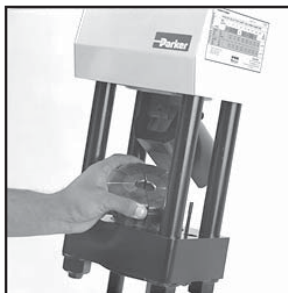
4. Place unitized die-train in bowl. See decal on crimper for proper die set. Note: Die sets are color coded by size.
