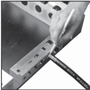
1. The Hose Insertion Depth fixture can be used to mark the insertion depth on the hose.
