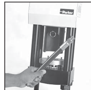
9. Release pump pressure and remove finished assembly.
