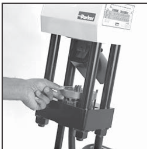
7. Place the die ring on top of the dies. See decal on crimper for proper die ring; Silver and Black.
